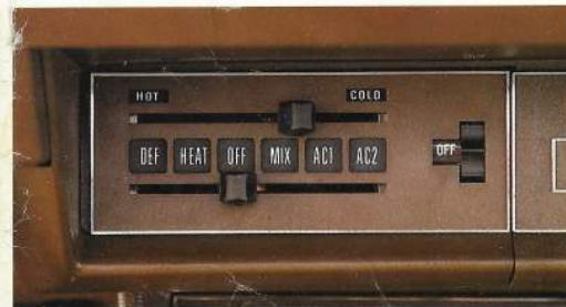
Air-conditioning control panel.
