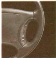
Steering wheel touch controls, standard on Series III models, allow you to operate the climate control and sound systems without removing your hands from the steering wheel or taking your eyes off the road.
