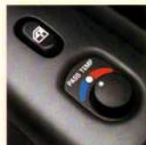
Dual-zone climate control lets the front passenger individually vary the temperature. (Available on Series II and Convertible.)
