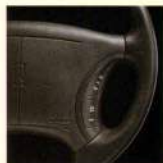
Touch controls let you adjust the stereo or climate control from the steering wheel. (Available on Series II and Convertible.)
