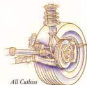
All Cutlass Supreme models feature four- wheel independent suspension with MacPherson front struts and four-wheel anti- lock disc brakes.
