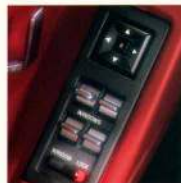
A power window lockout switch allows the driver to prevent rear windows from being opened by rear seat passengers.
