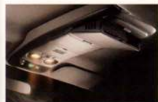
Silhouette's exclusive overhead console provides convenience like a concealed area for a garage door opener holder for sunglasses, dual map lights, and compass and outside temperature display.
