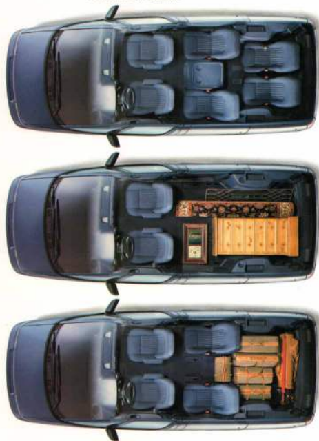
A number of flexible seating configurations provide a wide variety of easily created seating and cargo hauling options. Besides being removable, the last two rows of seats can also be folded down to become tables with handy cup holders.
