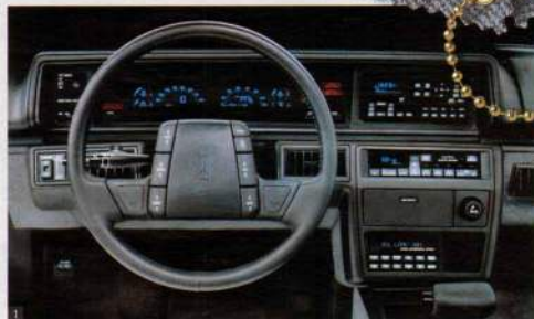
1. A leather-wrapped steering wheel with available touch controls that allow the driver to adjust climate and sound systems without ever releasing the wheel.
