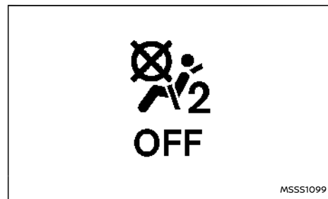
Front passenger air bag status light <OFF>
