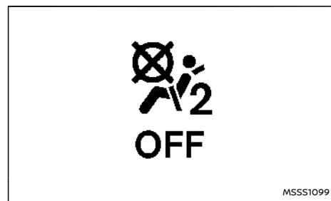
Front passenger air bag status light <OFF>
