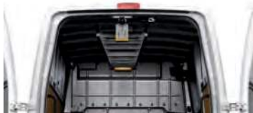
NV Cargo High Roof Cargo partition and interior overhead ladder keeper
