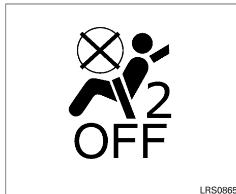
Front passenger air bag and status light
