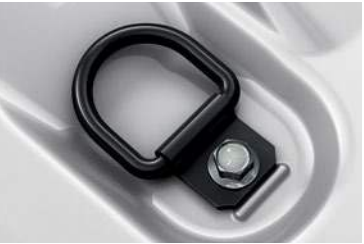
Six available floor-mounted D-ring tie-downs rated to 1,124 lbs.
