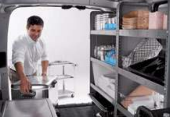
Integrated reinforced cargo-mounting points allow cargo racks, partitions and bins to be securely mounted, resisting loosening and tearing away from the interior wall. 1
