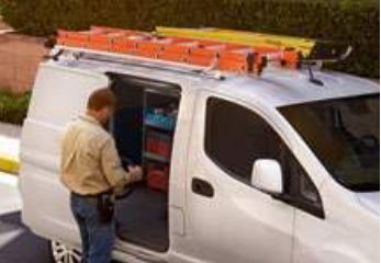
Integrated roof rack-mounting points help secure racks and reduce likelihood of rusting caused by drilling into sheet metal. 1
