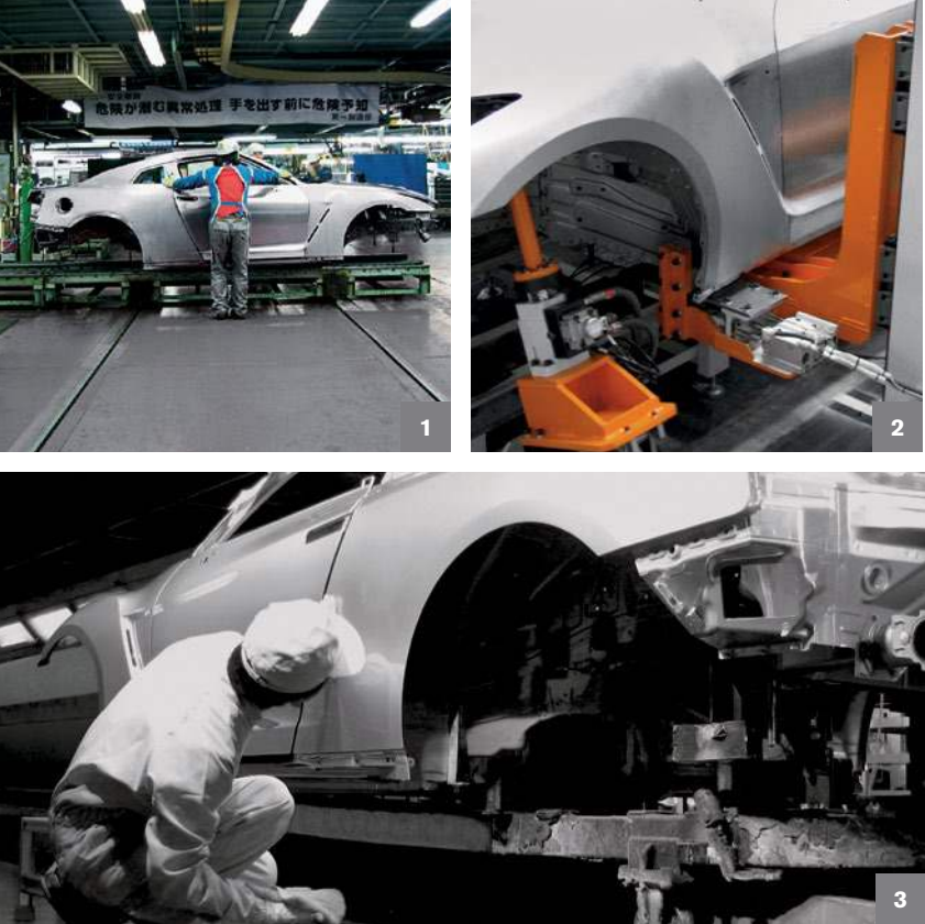
1_ Every GT-R receives a high degree of hand-assembly and finishing. 2_ Vibration testing, laser measurements, and comprehensive inspections by experienced specialists are performed to ensure long-term functionality and to maintain the highest levels of accuracy and precision during assembly. 3_ A craftsman uses both hand and eyes to inspect the body of a GT-R. To bring out any imperfections, three different light sources, including fluorescent, halogen and diffused flood lighting, are used to see various types of surface qualities in the paint as if it were at night, daylight or simply under intense scrutiny.
