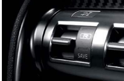
Transmission settings: R-Mode, Normal and Save
