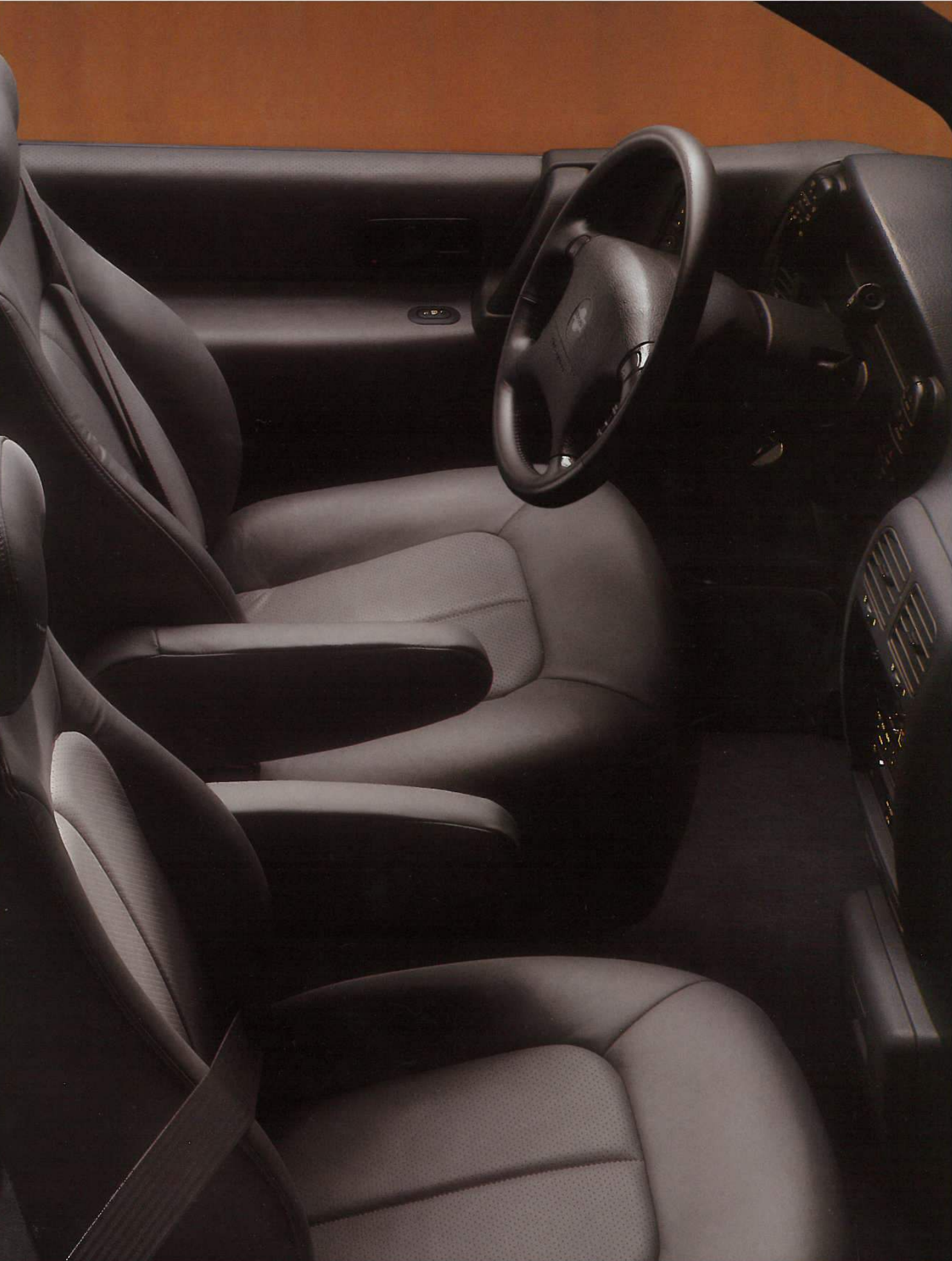
The seats have a firmer cushion and higher back than in traditional minivans, and the thigh cushion is specially angled, all to help prevent fatigue.
