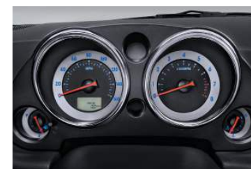
LED backlit gauges
