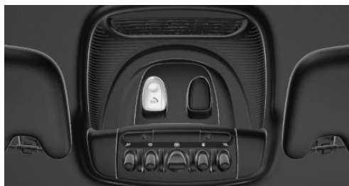
SOS button in the roofliner
