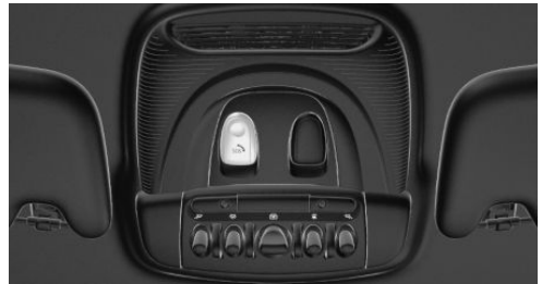
SOS button in the roofliner
