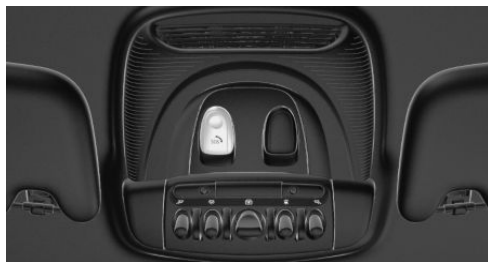
SOS button in the roofliner
