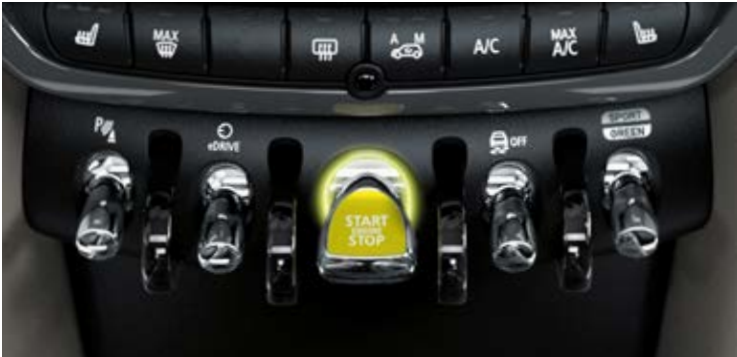
eDRIVE SWITCH. Three power modes to optimize your driving performance: Auto eDrive, Max eDrive and Save Battery.
