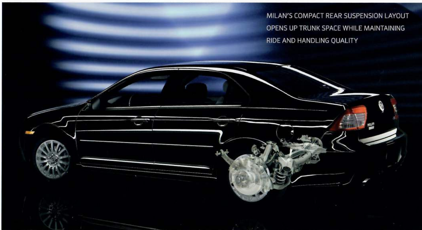
MULTI-LINK INDEPENDENT REAR SUSPENSION
