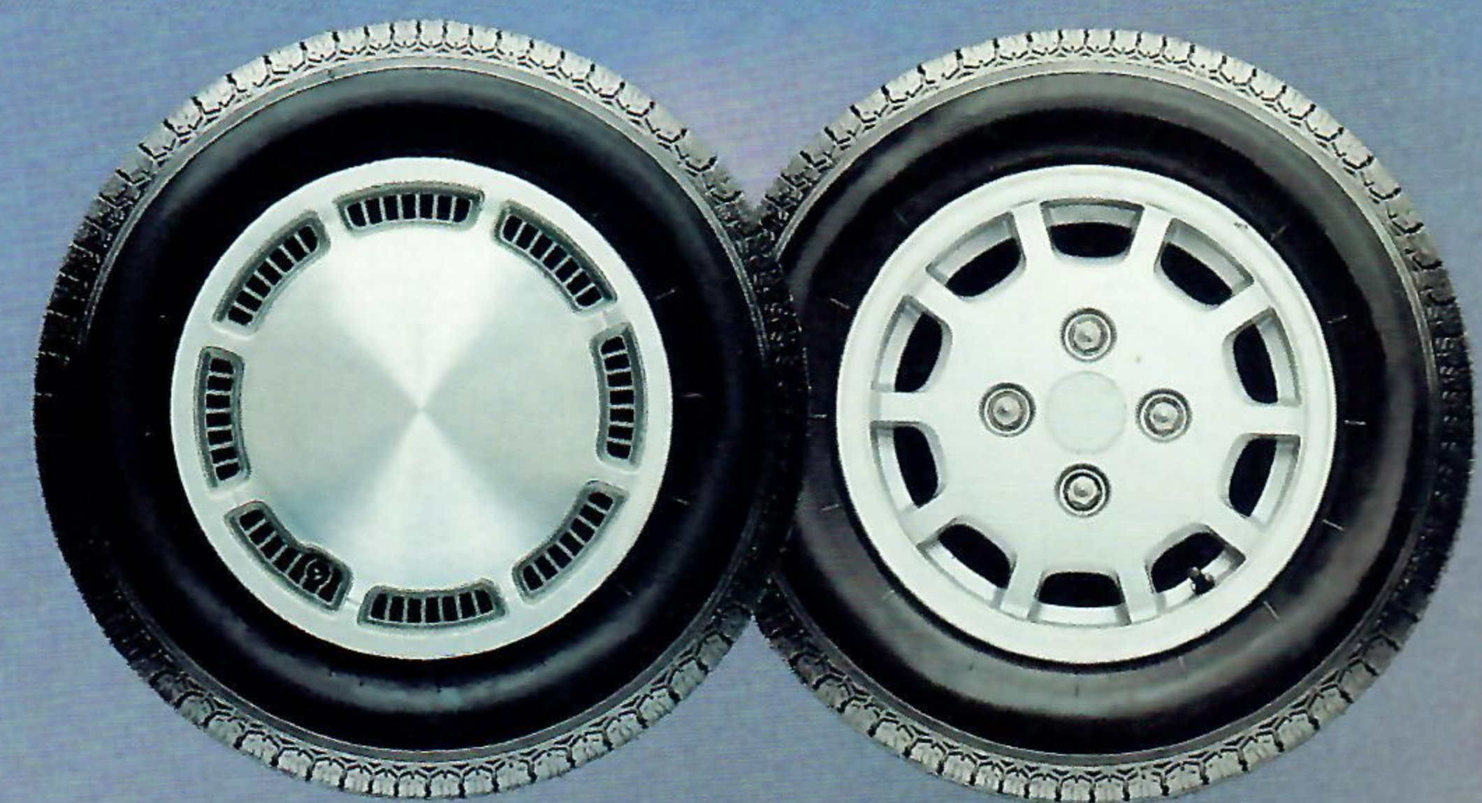
Satin finish wheel cover, cast-aluminum wheel.
