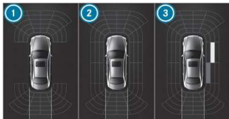
Parking Assist PARKTRONIC display: vehicles without a surround view camera
