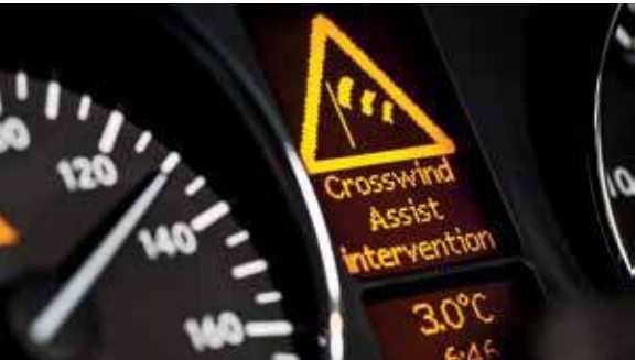
Crosswind Assist 2 can gently engage individual brakes to help quickly stabilize your Sprinter Van and boost safety in strong, gusting crosswinds. This standard feature helps ensure that your van remains in its lane at highway speeds.
