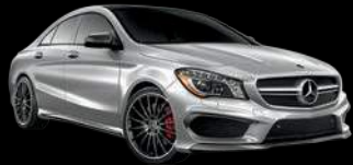
AMG CLA 45 Coupe 375 hp @ 6,000 rpm 350 lb-ft @ 2,250–5,000 rpm
