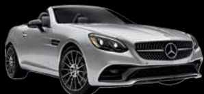
AMG SLC 43 Roadster 362 hp @ 5,500–6,000 rpm 384 lb-ft @ 2,000–4,200 rpm
