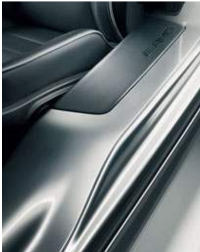
Door sill panels in vehicle colour with nappa leather insert and embossed AMG lettering
