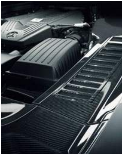
AMG carbon-fibre engine compartment cover
