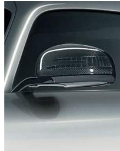
AMG carbon-fibre exterior mirrors
