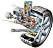
1982 Multilink rear suspension
