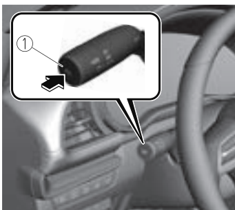
1. High beam control switch
