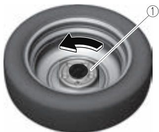
1. Spare tire hold-down bolt
