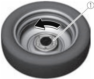
1. Spare tire hold-down bolt
