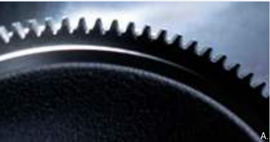
A. The MX-5 Miata utilizes an ultralight flywheel to enhance the engine’s free-revving performance and improve its responsiveness. B. Friction-reducing, molybdenum-coated pistons plus a high-compression ratio help the current MX-5 Miata engine generate 17% more horsepower than the previous generation’s powerplant. C. A limited-slip differential and Dynamic Stability Control with Traction Control System are available on select MX-5 Miata models.
