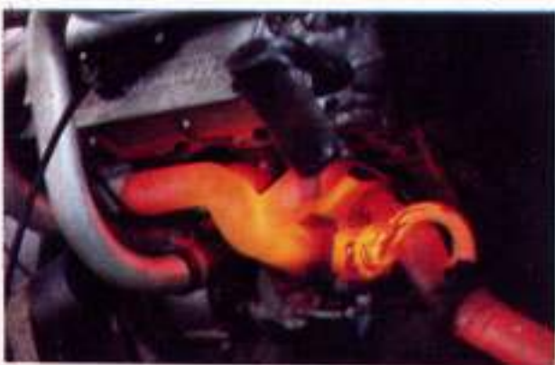
Biturbo engine on the dynamometer during extremely heavy endurance tests at maximum power and speed
