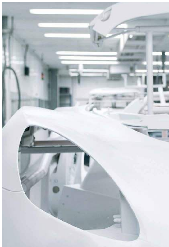
Right: Elise composite bodywork ready for paint
