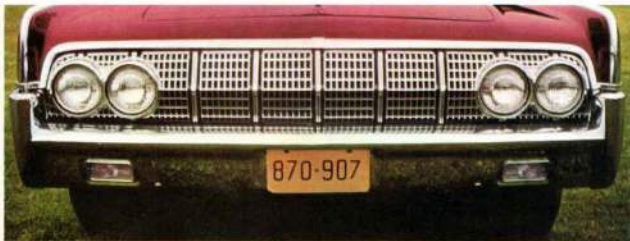
The classic fender guard and unadorned fender line. Modification in the sculpture of the front grille. The horizontal setting of its twin headlights.
