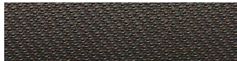
Carbon Fiber with Copper Wire Weave finisher
