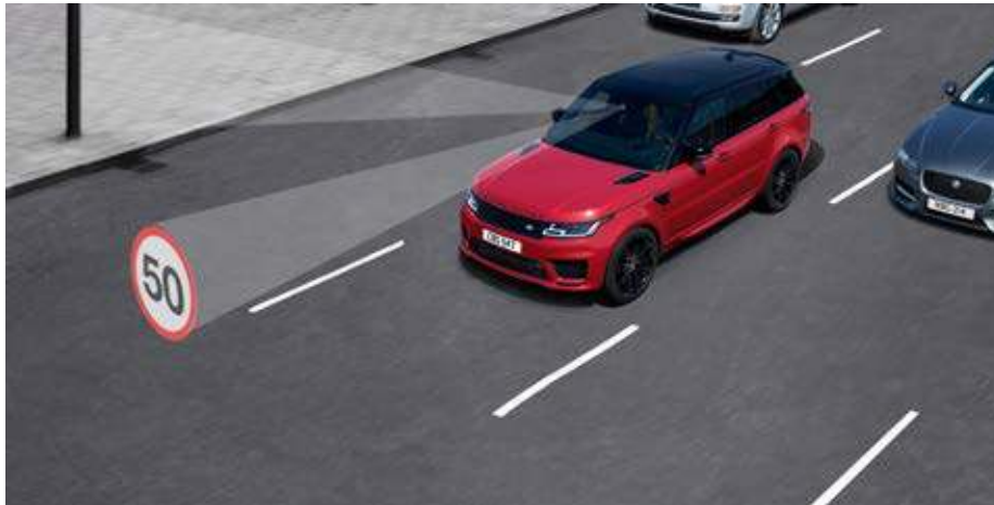
Traffic Sign Recognition with Adaptive Speed Limiter
