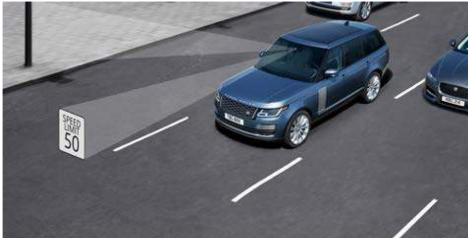
Traffic Sign Recognition with Adaptive Speed Limiter
