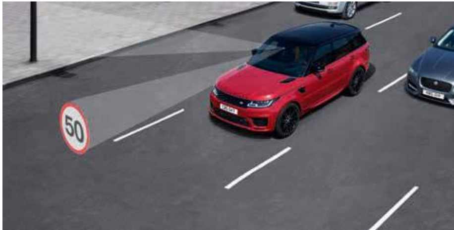
Traffic Sign Recognition with Adaptive Speed Limiter
