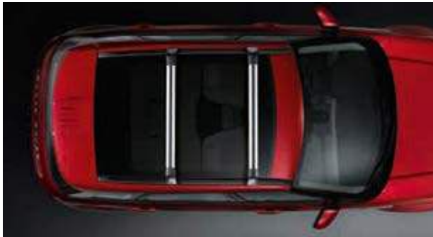
Crossbars* Δ VPLVR0073 Silver finish, adjustable position cross bars for vehicles fitted with roof rails. Aerodynamic profile designed to minimize drag and noise. Lockable for security and incorporating a T-slot to carry the Land Rover roof mounted accessory range. Vehicle height when fitted: 5.64ft. Maximum permissible load capacity 158lbs**.
