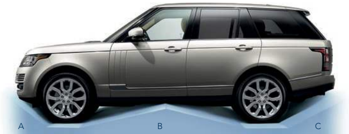
Obstacle Clearance Off-road height 11.63 inches Standard ride height 8.68 inches
