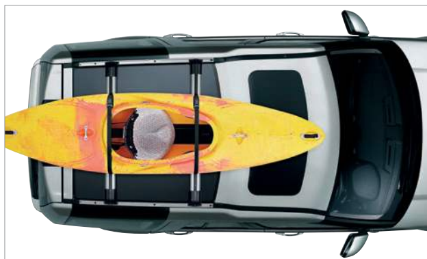
Aqua Sports Carrier** VPLGR0107 Carries one surfboard or sailboard and mast, or one canoe or kayak. Includes lockable multi-purpose holder to carry a mast, oars or paddles. Tilts to facilitate easy loading and unloading. Maximum payload 99lbs 1 .
