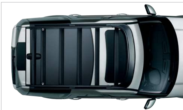
Expedition Roof Rack** CAB500021PMA Vehicle must be fitted with a Black Finish or Bright Finish Short Roof Rail Kit CAB500120PVJ/CAP500090. Vehicle height when fitted 83 inches at normal ride height. Maximum payload 120lbs 1 .
