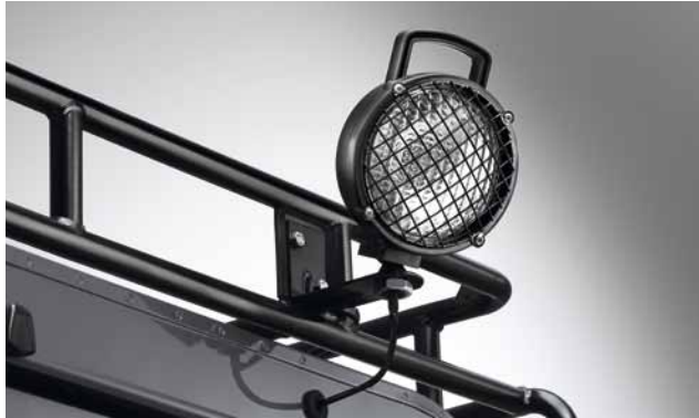
Worklight RTC8921AA Enables your Defender to provide floodlight style illumination when working in reduced lighting conditions. Fits both 90 and 110 models. Switches, cables and brackets are supplied in the kit.
