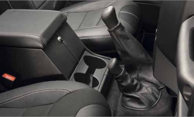
Black Leather Hand Brake, Gear and Transfer Lever Gaiters VPLDS0258 Grained Leather Gaiter covers detailing ebony coloured twin stitch features.
