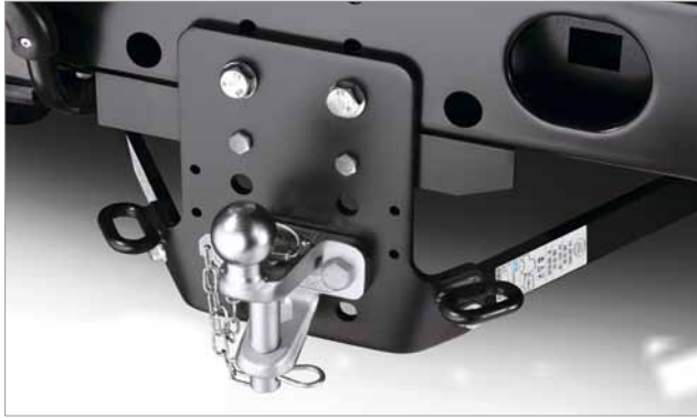
Combination Tow Ball/Jaw Unit* LR008244 50mm tow ball and jaw combination for increased towing versatility and a 3,500kg capacity. Tow Jaw*** KNB100640 – (not shown) With a 3,500kg capacity.
