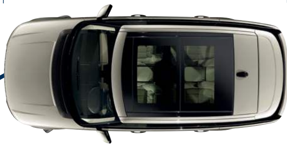
Standard overall length 4,999mm/196.8 inches (Long Wheelbase 5,199mm/204.7 inches)
