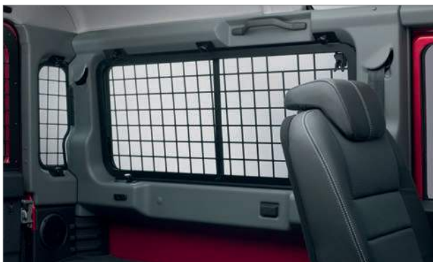
Interior Window Guards – Side Windows VPLDS0247
