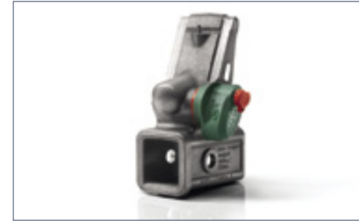
Quick Release Tow Hitch Receiver LR040248 Lockable for security. Easily removed. 1.9 inches/48mm Tow ball, height 15 inches/381mm from ground. 7,716lbs/3,500kg trailer load capacity (551lbs/250kg trailer nose load).
