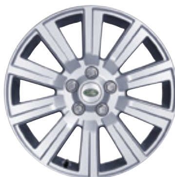
19 INCH TEN-SPOKE TIRE SPECIFICATION: 255/55AT STANDARD ON LR4 HSE
