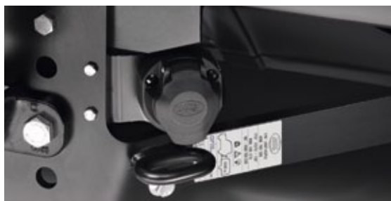
13 Pin Towing Electrics* LR005919 European style towing electrics, capable of supplying all trailer rear lighting and interior equipment power; including fridge feed and battery charging.
