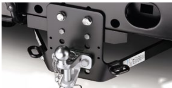
Combination Tow Ball/Jaw Unit** LR008244 50mm tow ball and jaw combination for increased towing versatility and a 3,500kg capacity.
