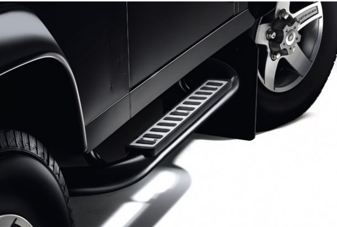
Side Protection Runners Black Finish – Defender 90 – LR008379 Black Finish – Defender 110 (not shown) – LR008375 The sturdy steel design enhances the appearance of your Defender as well as helping to ease entry and exit. The moulded rubber footgrips help to ensure non-slip stability.
