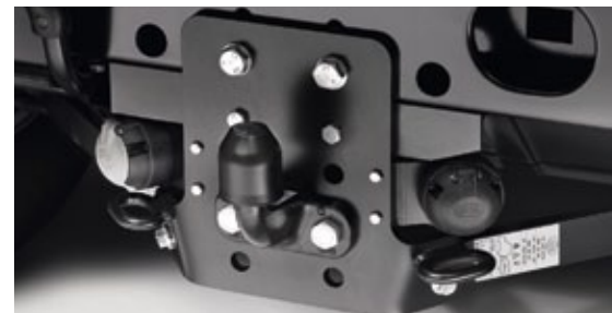
'S' Type Towing Electrics* (shown above, left-hand side) – LR005921 For use when additional trailer power is required. Capable of supplying interior lighting and equipment power including fridge feed and battery charging. Please note: Not compatible with standard fitted 12N sockets. Must be used in conjunction with 'N' Type Towing Electrics LR005920.
