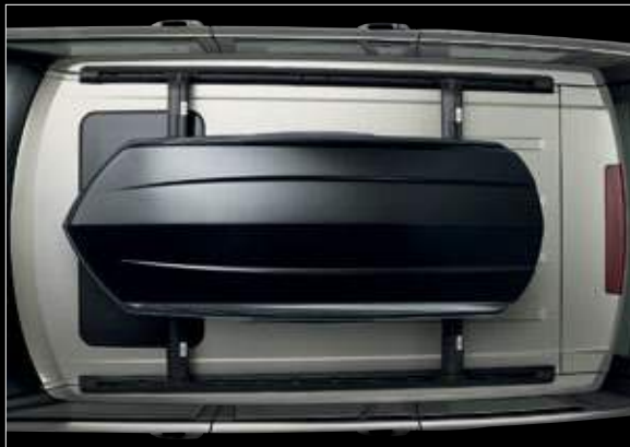
Sports Box* VPLVR0061 Gloss Black finish. Can be mounted on either side of the vehicle for curbside opening in any country. Internal retention system for skis or other long loads. Lockable for security. External dimensions: 81.1 inches long, 33.1 inches wide, 13.4 inches high. Volume 111 gallons. Load capacity 165.3lbs.
