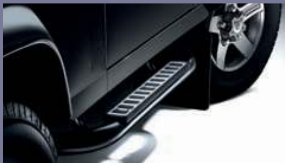
Side Protection Runners – New Style Black Finish - Defender 90 - LR008379 Black Finish - Defender 110 (not shown) - LR008375 The sturdy steel design enhances the appearance of your Defender as well as easing entry and exit. The moulded rubber footgrips ensure non-slip stability.
