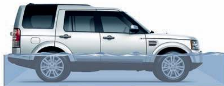
Wading Depth Maximum wading depth 27.56 in. (700mm) (with air suspension raised) Normal wading depth 23.62 in. (600mm)
