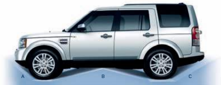
Off-road Geometry A B C Approach Angle 37.2° Ramp Break Over Angle 27.9° Departure Angle 29.6° Off-road ride height (air suspension)
