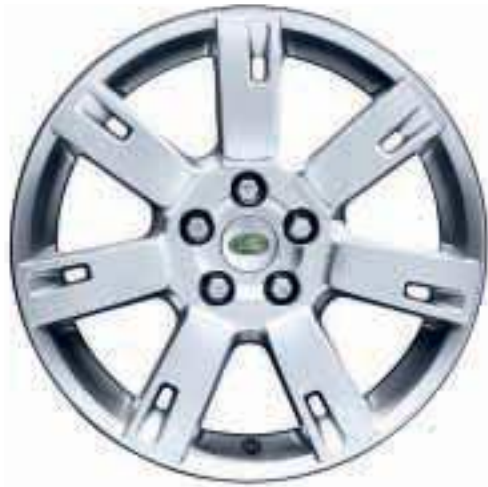
LR4 19 INCH 7-SPOKE ALLOY WHEELS Tire Specification: 255/55 AT
