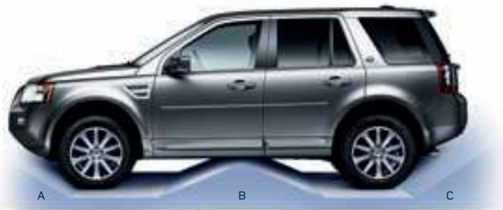
Off-road Geometry A B C Approach Angle 29° Ramp Break Over Angle 21.5° Departure Angle 32°
