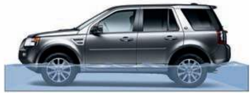
Wading Depth Maximum wading depth 19.7 inches/500 mm
