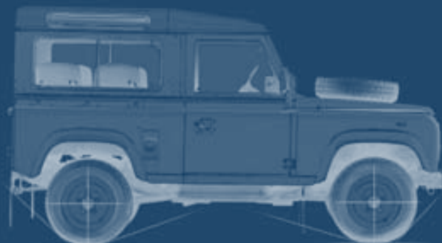
'90' Station Wagon (1984-1990) 1984 Leaf springs upgraded to coil springs. One-piece windscreen introduced. Wind-up front windows replace sliding windows. Polyurethane wheel arches introduced to accommodate wider track.
