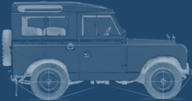
Series II Station Wagon (1958-1961) 1958 Side windows enlarged. Sills introduced to obscure exhaust and powertrain. Fuel filler cap moved from under driver's seat to behind driver's door (RHD).
