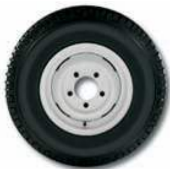
STANDARD STEEL WHEEL 90/110 5.5F X 16, 140 X 406
