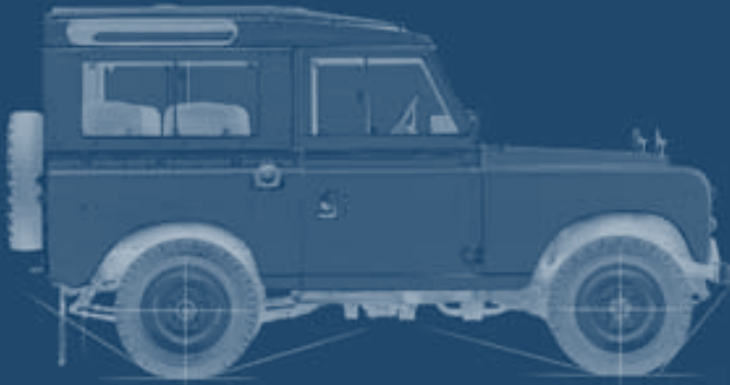
Series III Station Wagon (1972-1984) 1972 Air intake on wing for heater added. 1981 Improved seating introduced on County models.
