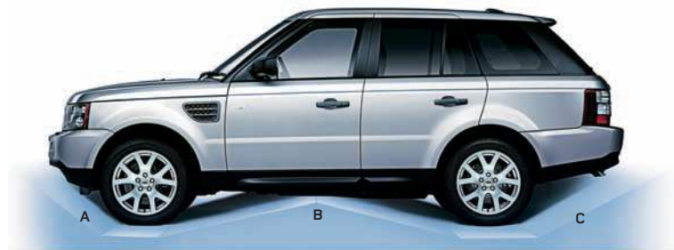
Obstacle Clearance Ground clearance off-road height 8.9 inches (227mm) Standard ride height 6.8 inches (172mm)
