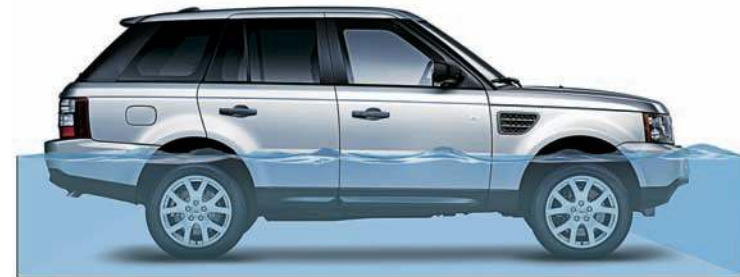
Wading Depth Maximum wading depth 27.6 inches (700mm)*
