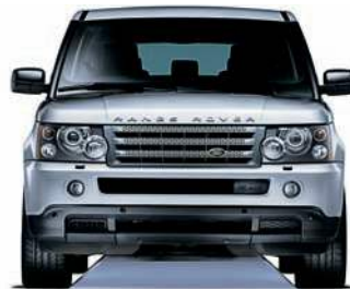
Obstacle Clearance Ground clearance off-road height 8.9 inches (227mm) Standard ride height 6.8 inches (172mm)
