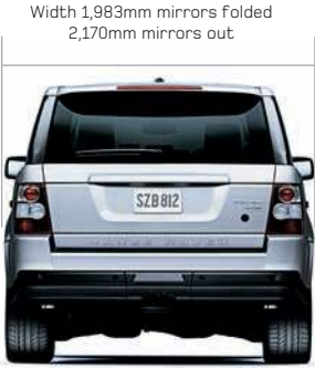
Rear wheel track 63.5 inches (1,612mm)
