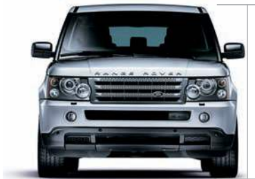
Maximum vehicle height Standard mode – with Satellite Antenna 70.4 inches (1,789mm) Access mode 68.3 inches (1,734mm)
